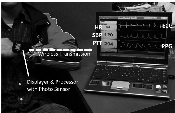
Fig. 3. An h-shirt-based wearable intelligent systems for e-Health (WISEs) prototype developed in our research center for monitoring electrocardiogram, photoplethysmogram, and cuff-less blood pressure based on the estimation of pulse transit time [13].
