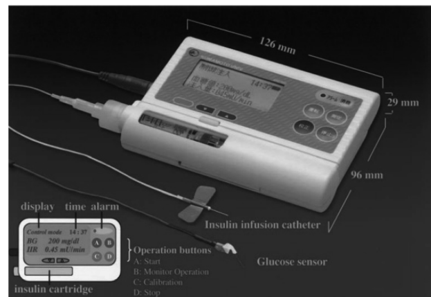
Fig. 2. A wearable artificial endocrine pancreas with a needle-type glucose sensor [28].
