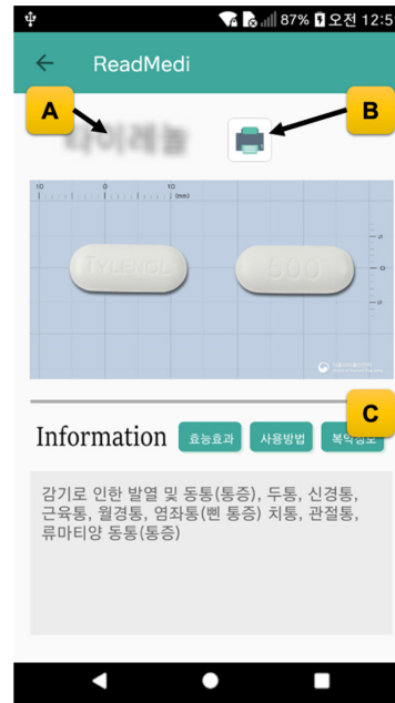
Fig. 7. Screenshot of the mobile application. 'A' is a name of the recognized medicine, 'B' a print button for braille embosser and 'C' an efficacy and safety information of the recognized drug.
