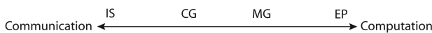
Fig. 1. Four representative parallel jobs and their characteristics according to computation and communication. IS: integer sort, CG: conjugate gradient, MG: multi-grid, EP: embarrassingly parallel.
