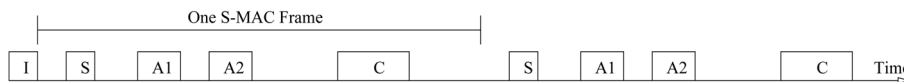
Figure 3. The events in the S-MAC frame (I Event: the initialization event, S Event: the sample event, A1 Event: the tx application event, A2 Event: the rx application event, T Events: a series of tx byte events and rx byte events, C Events: a series of S-MAC clock events).
